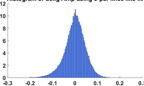
■ This figure shows the distribution of the deviation for the amplitude using 5-par Knee-like fit, where we found that the RMS for Amp ~ 0.05 and for Q ~ 0.1
