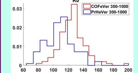
Distribution of the parameter  $R_0$  for proton-Helium (blue) and Carbon-Iron (Red) two samples for energy from 300-1000 TeV at angles 0-25. We can see that using  $R_0$  parameter we can separate between heavy and light nuclei with a good accuracy.
