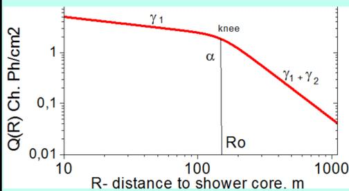
$R$  is the distance from the shower axis;  $a$ ,  $\gamma_1$ ,  $\gamma_2$ ,  $R_0$  and  $\alpha$  are the parameters of the Cherenkov light LDF
