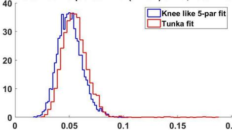
■ This figure shows the Root-Mean-Squared Error (RMSE) which characterizes the accuracy of fitting for every event. It was calculated from these equations:
