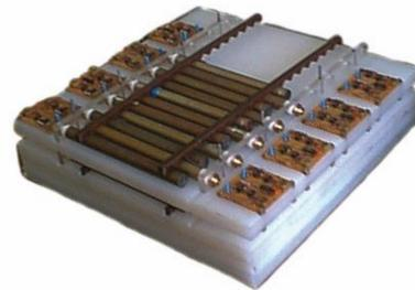
Fig. 3. The PAMELA neutron detector
