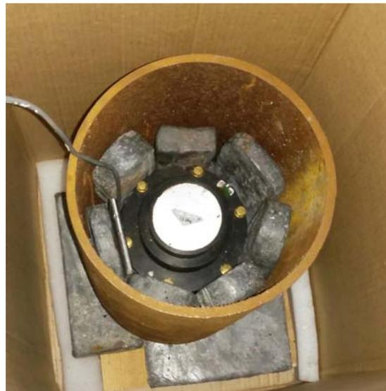
**Fig. 2. The Barentsburg scintillation gamma-detector with steel and lead shells.**
