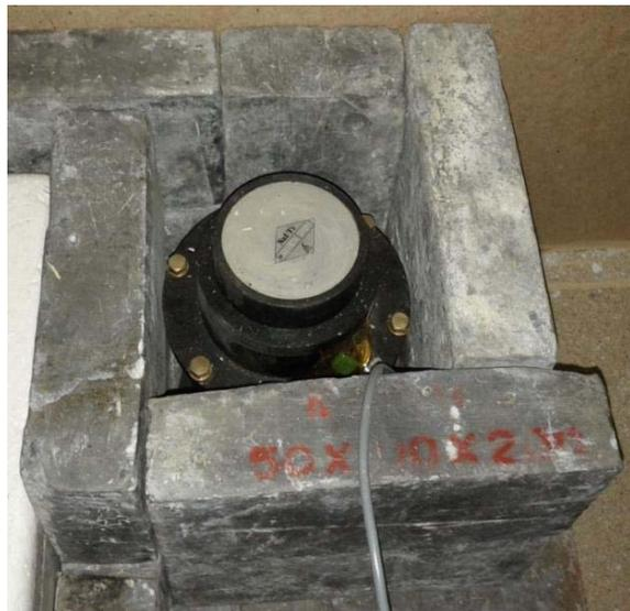
**Fig. 1. The Apatity scintillation gamma-detector with lead shell.**
