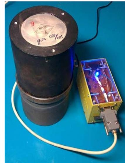
**Fig. 3. The Rostov-on-Don scintillation gamma-detector with microcontroller-based registration system.**
